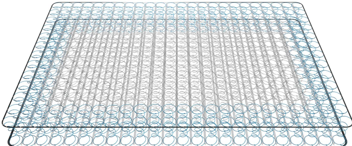
ProZone® is a programmable Bonnell innerspring system that uses fully automated, computer-controlled zoning technology to produce coils of varying diameter and firmness level in specified zones.
